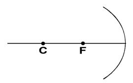
Case 4: The object is located at the focal point (F)
