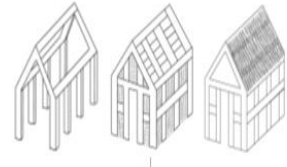
Wattle and Daub House Construction
