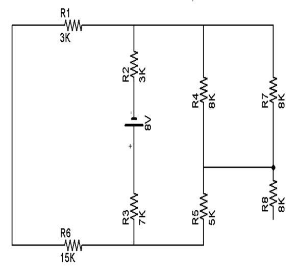
Note one end of R8 is not connected, meaning that no current flows as it is not a complete circuit. Therefore, according to Ohm's law, V8 must be what?
