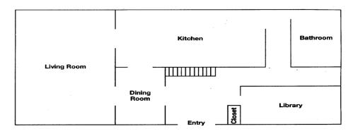
Above is the first floor plan for a new house. The plan is drawn to a scale of 0.5 in. : 4 ft. Use a ruler to measure the necessary dimensions.
